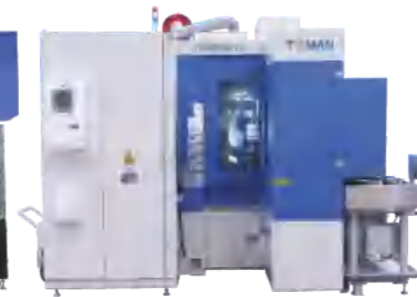
滚棱一体复合机 Gear Hobbing Machine with Integrated Chamfer Hobbing Unit
