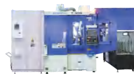
滚倒一体复合机 Gear Hobbing Machine with Integrated Chamfering Station
